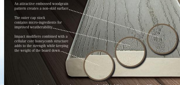
In our co-extrusion process, the UV inhibitors and modifiers for weatherability and heat reflection are concentrated in an outer layer while, stabilizers and impact modifiers for durability and strength are blended into the inner core of the product.
